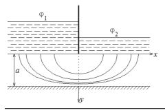
Filtration flow diagram for the point dam with an aquitard
